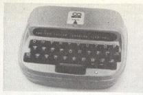
MIGET (miniature interface general-purpose economy terminal) provides keyboard entry and simultaneous 32-char display output compatible with all microcomputer and microprocessor systems using RS-232-C interface and ASCII code. The 8 x 10 x 3" (20 x 25 x 7.6-cm) terminal weighs 4 lb (1.8 kg). Features include eight selectable baud rates from 110 to 9600, complete TTY compatibility, and optional self-contained memory system and acoustic coupler. Micon Industries, 252 Oak St, Oakland, CA 94607.
