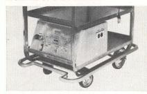
PEP is designed to provide clean uninterruptible electric power to sensitive electronic equipment, and to protect this equipment from circuit fluctuations caused by voltage changes, overloaded lines, frequency shifts, or power failure. Std models output 100, 250, or 500 VA, and are complete with stainless steel cart. The system operates from internal batteries or from any std ac line, or from both. Marine Electric RPD, Inc, 178 National Rd, Edison, NJ 08817. Circle 250 on Inquiry Card
