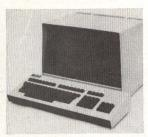
A Teletype<sup>™</sup>-compatible display terminal with roll or page mode of operation utilizing the ASCII code set, model 200 features 80 x 24-char display, 9 x 9 dot matrix, character mode transmission, RS-232-C and 20/60-mA current loop interface, and 16 switch-selectable data rates up to 19,200 bits/s. The
