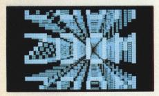
virtuoso display. You'll see zoom and pan, area shading, pattern definition, rubber band line, scientific plotting and graphics text composition. Having independent memories for graphics and alphanumerics, you can do auto-plots with or without words and figures on the screen.
