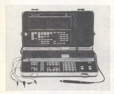
Portable MicroSystem Analyzer contains all facilities required to monitor and control fault isolation process in a 6800 or 8080 microprocessor-based system under test. Signature analysis and in-circuit emulation combine to provide capabilities that are more powerful than those of either approach used alone
