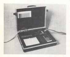
able from RCA Solid State Div, Rte 202, Somerville, NJ 08876, the tool is housed in an attache case containing built-in keyboard, display, and status indicator lights, as well as software debugging routines. A self-test card simulates a user system to verify and assure the monitor's operation.
